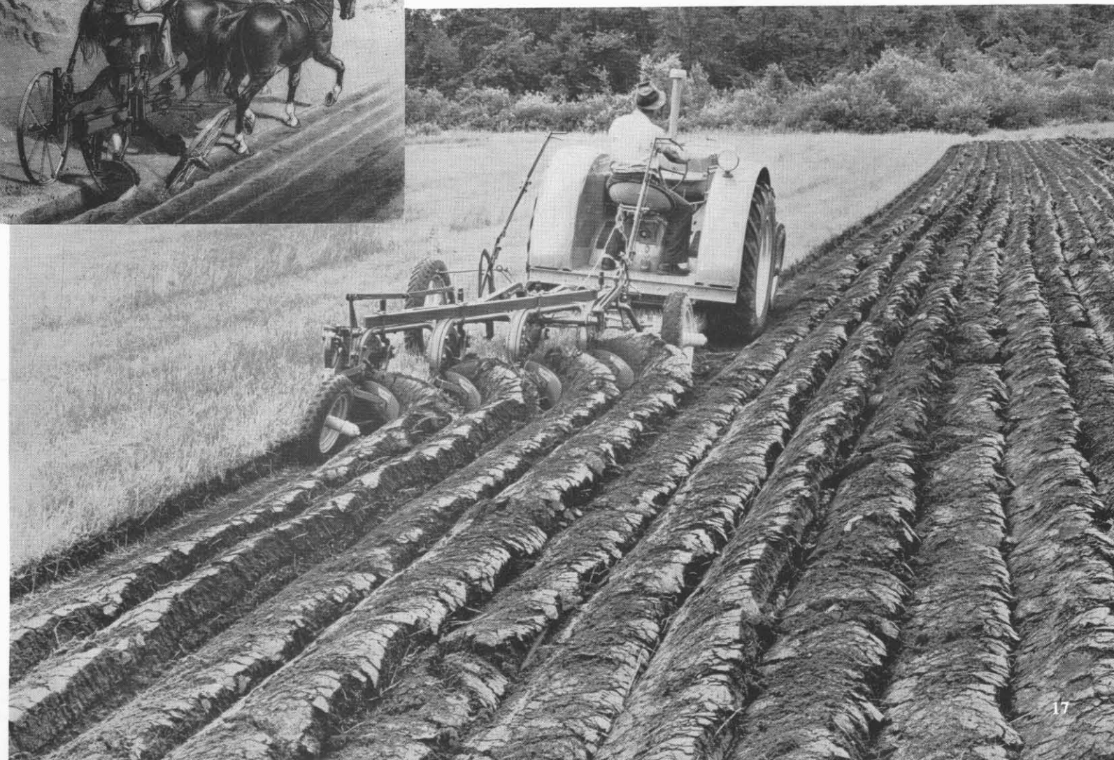
In 1875 a farmer needed three horses to draw a one-share sulky plow with oblique wheels (left). Today a tractor easily pulls four shares.
