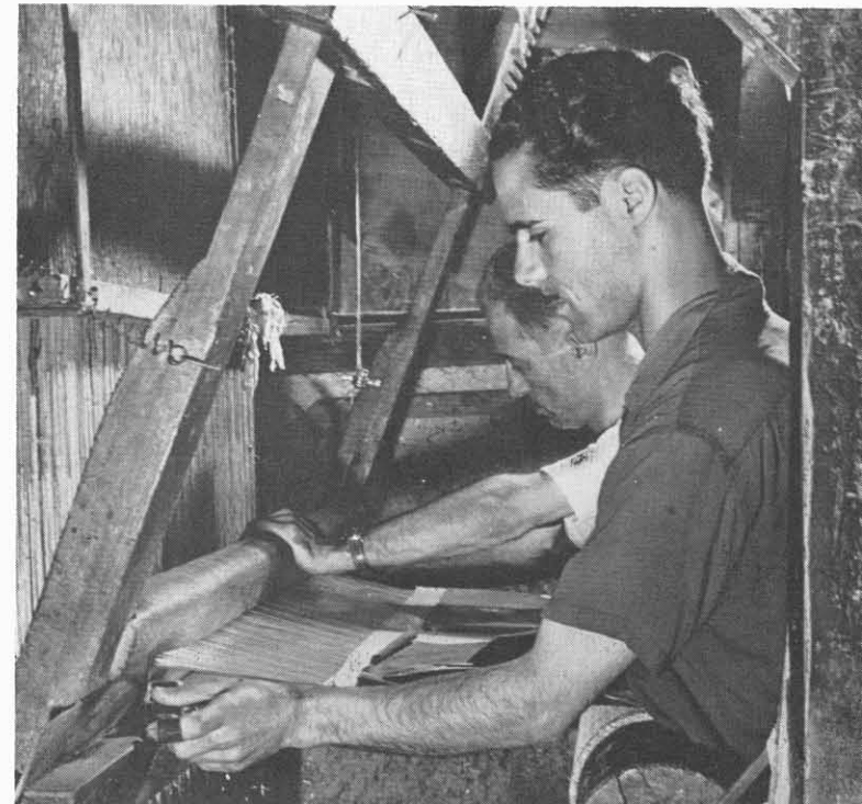
Operators toss the woof shuttle (carrying design color) back and forth through the warp. The material (produced an inch an hour) is kept tightly drawn by the pressure board in front.
