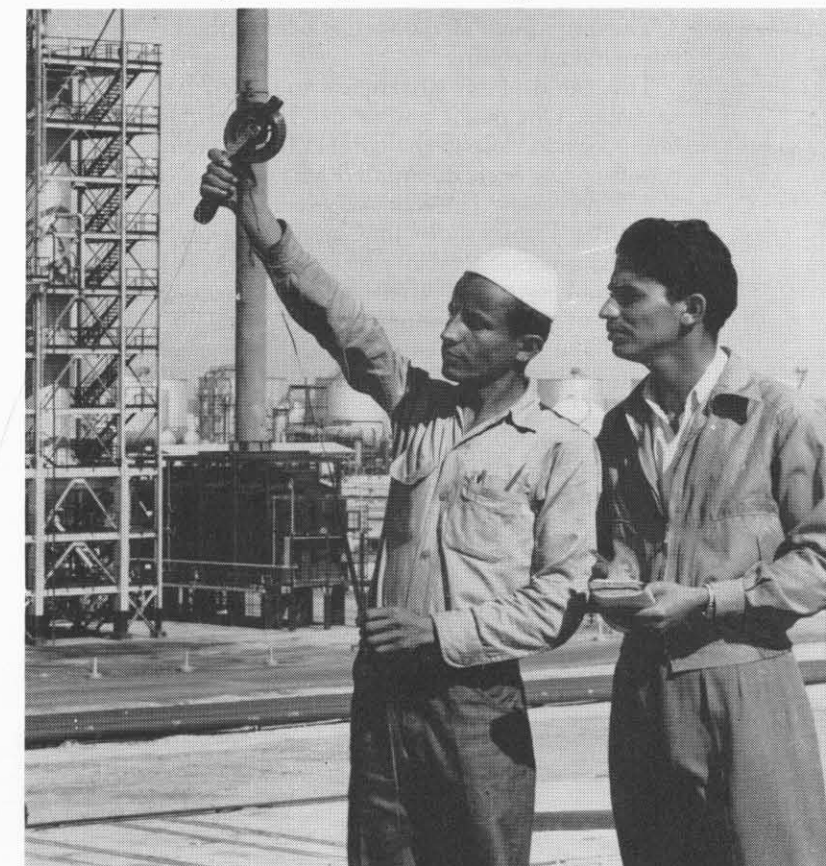
Gaugers from Aramco and Saudi Arab Government measure the volume of the crude oil to be refined at Ras Tanura.
