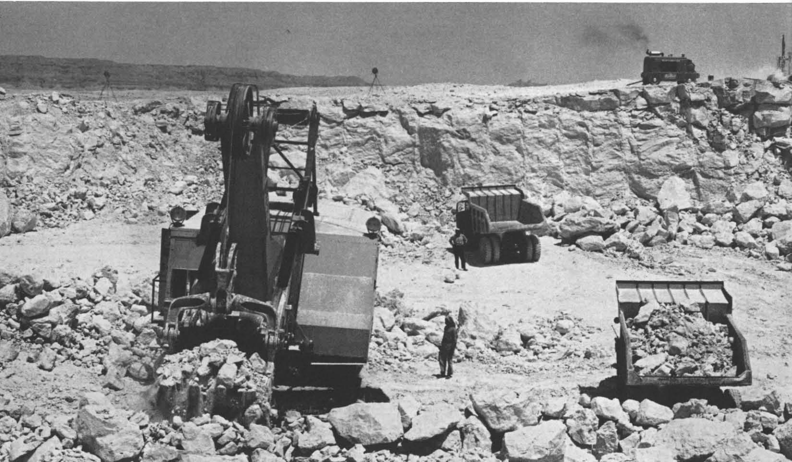
A 100-ton power shovel bites into the blast-loosened limestone, which is 98 per cent calcium carbonate and ideal for cement manufacture.
