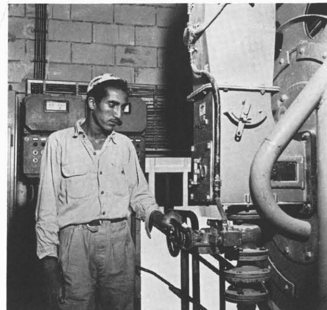
A technician controls temperature of gas burner in drying unit.
