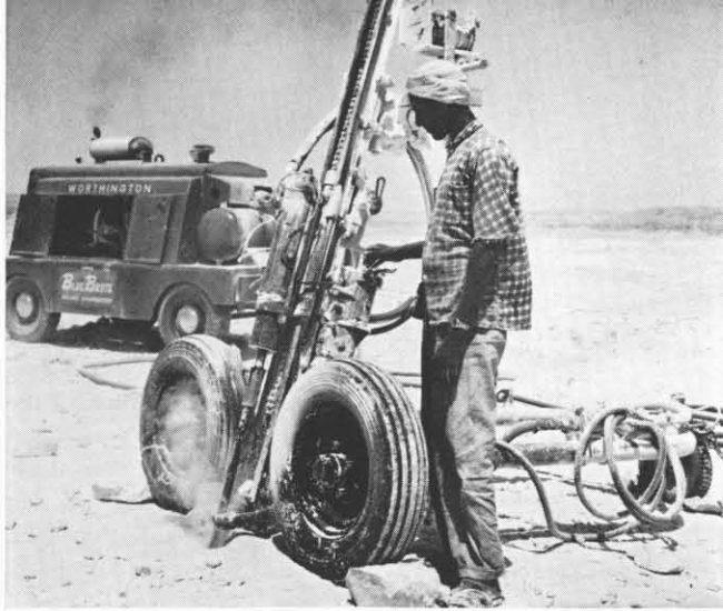
At a quarry nearby the cement factory, a compressed air drill prepares holes for the explosive charges that loosen limestone.
