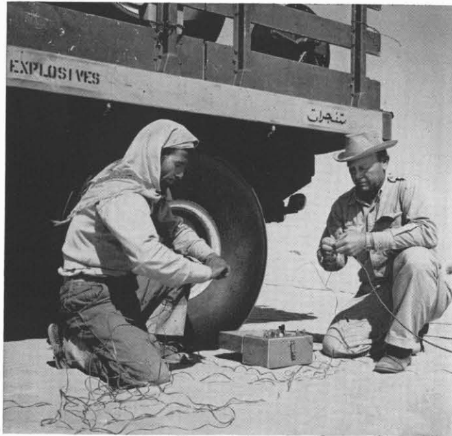
A shooter (left) prepares detonating equipment that will set off dynamite charge. Shock waves from the subsurface blast will be recorded by sensitive geophones known to seismographers as jugs
