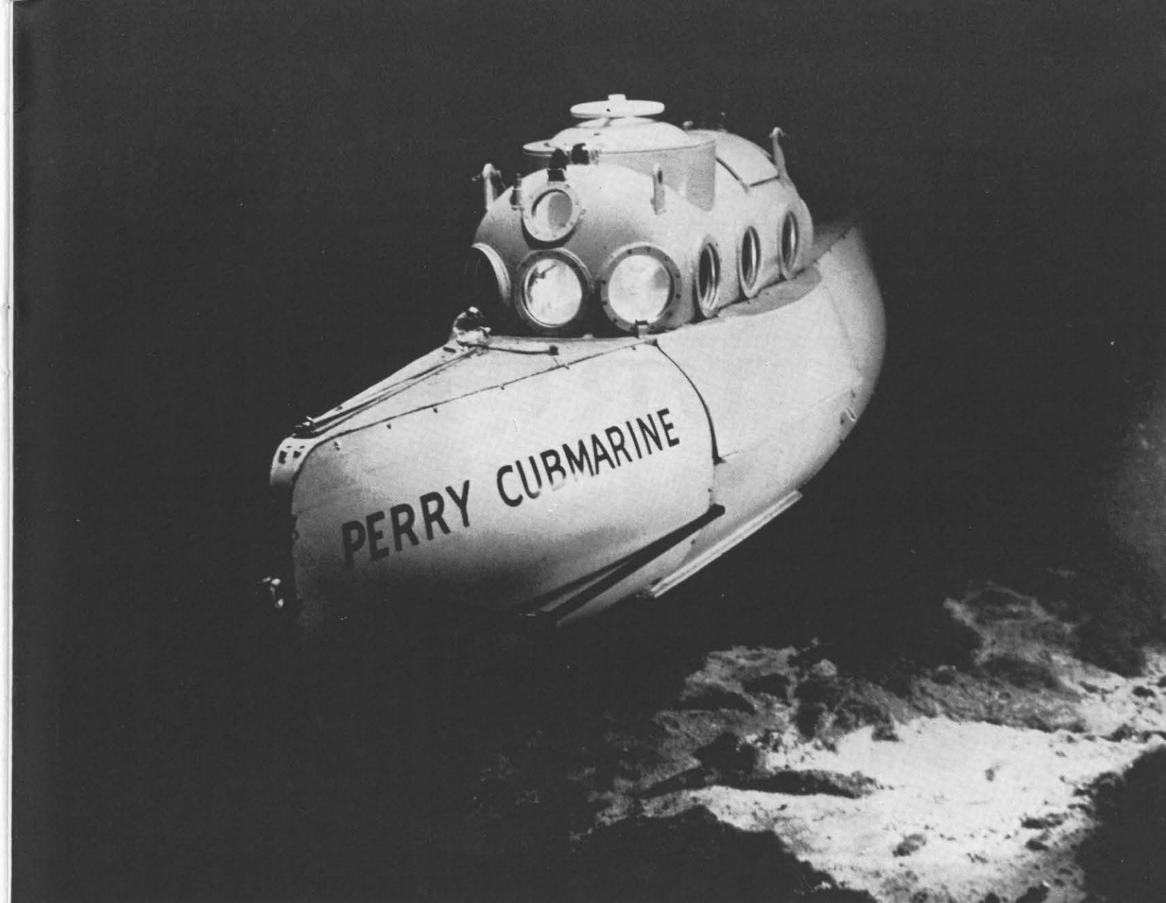
Newly developed Cubmarine, 20 feet long, has two-man crew for exploration, physical-biological studies, salvage, and underwater inspections.
