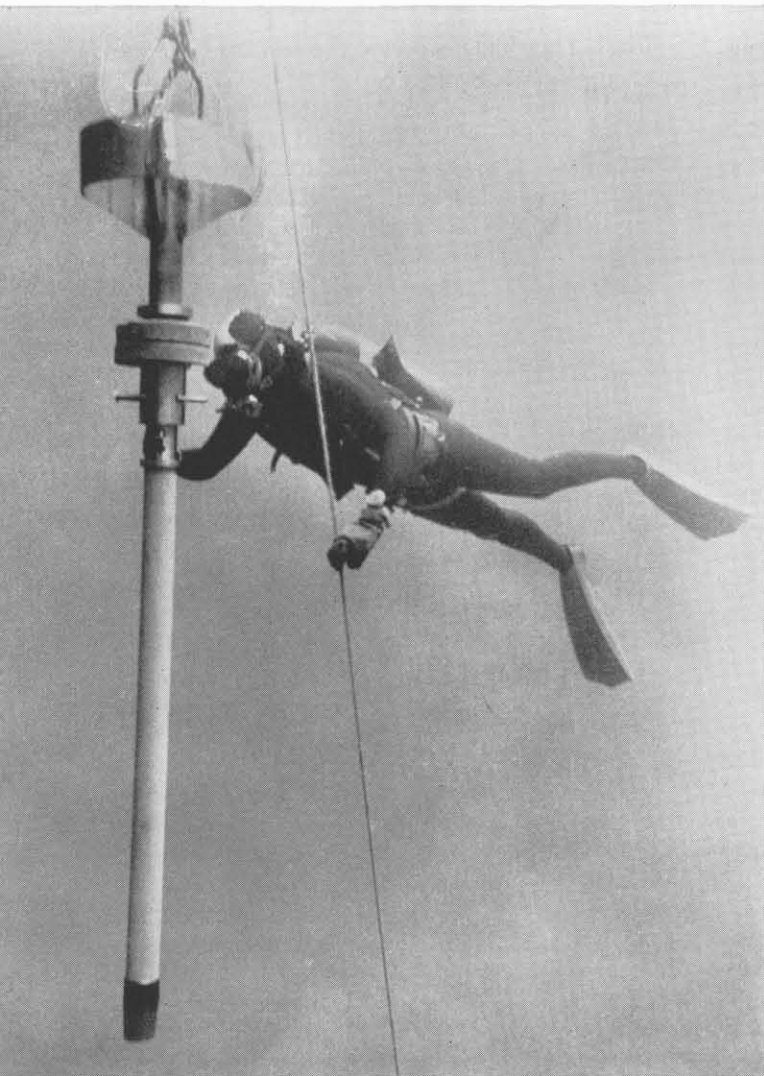
Sea-bottom corer, plunging to ocean floor as scuba diver aids its descent, extracts five-foot-long core of bottom. Cores are then analyzed in laboratories in connection with undersea mining surveys, tests for underwater construction, and geological and biological examinations. An underwater sled (below) helps map sea floor contours. On sled are a depth sensor and an inclinometer. Information is sent by communication-towing cable to recording instruments aboard the ship which tows the stainless steel sled.
