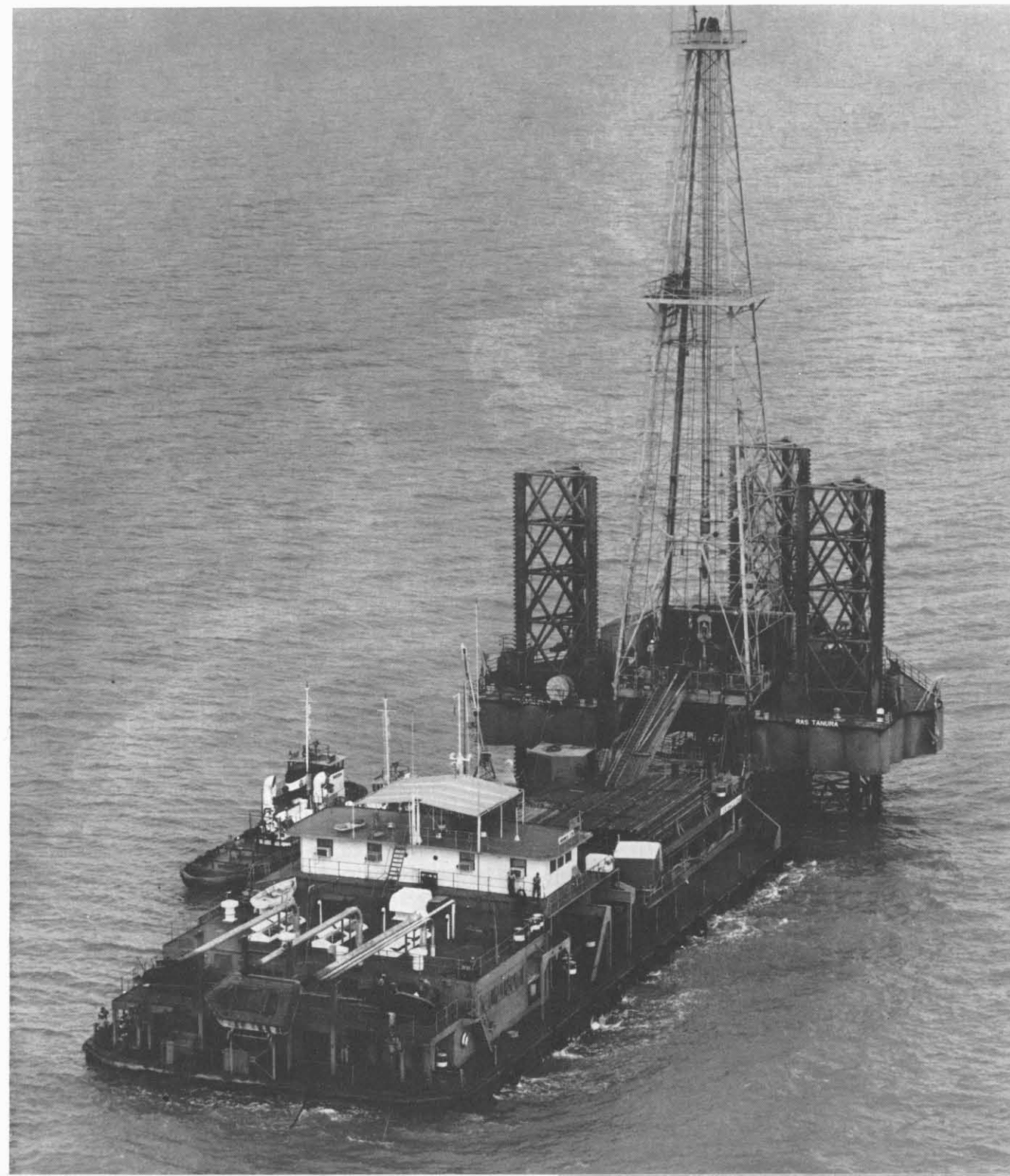
With her legs resting on floor of the Persian Gulf, AMDP-1 is being readied for installation of drilling rig on the platform. Barge 136 (below), popularly known as Queen Mary, works with AMDP-1 at Manifa field. After nearly 10 years' service Queen Mary was converted in 1963 to pipelaying and heavy-lift barge.
