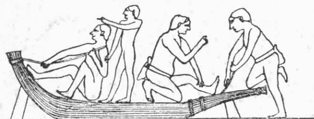
Long before they began to employ wood in boatbuilding, craftsmen along the Nile River tied together three bundles of papyrus reeds.
