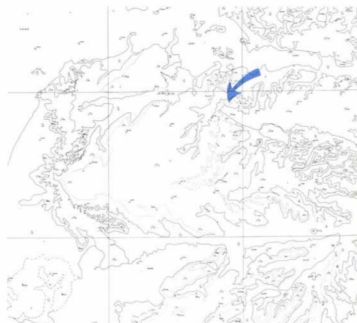
Interpretation of aerial photographs and geological data collected by surface mappers on the ground went into the making of this map, which clearly shows dividing lines between the various geological formations. Letter symbols scattered over the surface of map indicate individual geological formations. Visual comparison of similar configurations shown on previous picture and this one, covering the same area, shows that geological formation boundaries frequently follow escarpments and other terrain features.
