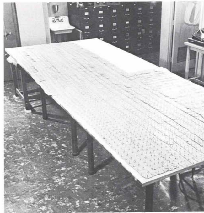
A map projection, consisting of lines of latitude and longitude, is drawn and constructed on a large flat surface. On the map projection, map-makers lay down a slotted pattern consisting of hundreds of individual stiff cardboard templates, adjusting them to strategically-located fixed ground control stations plotted according to their geographic coordinates.
