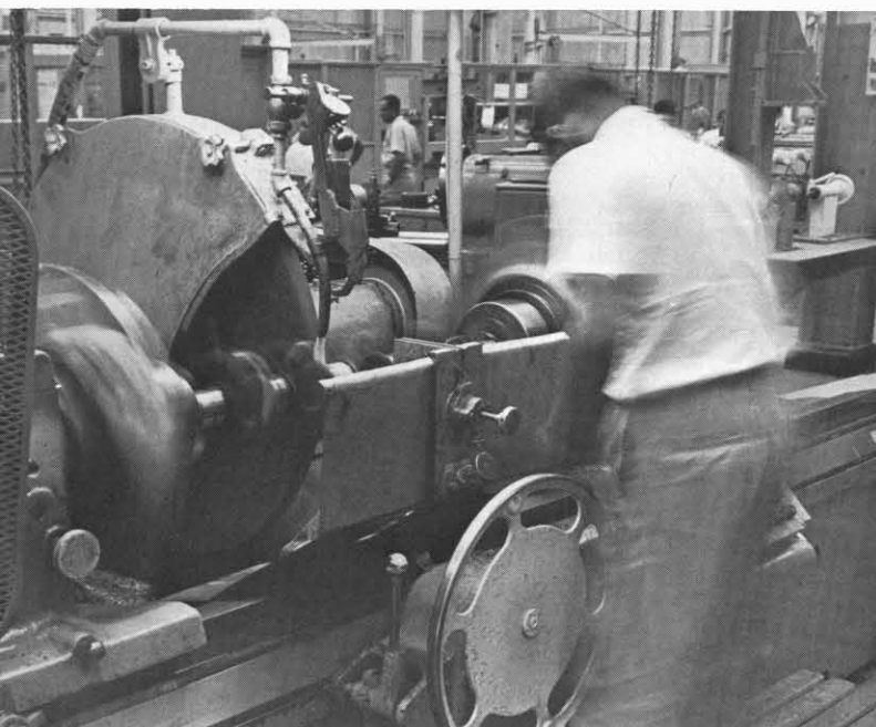
Machinist 'Abd al-Hamad guides a huge emery wheel to regrind a crankshaft.
