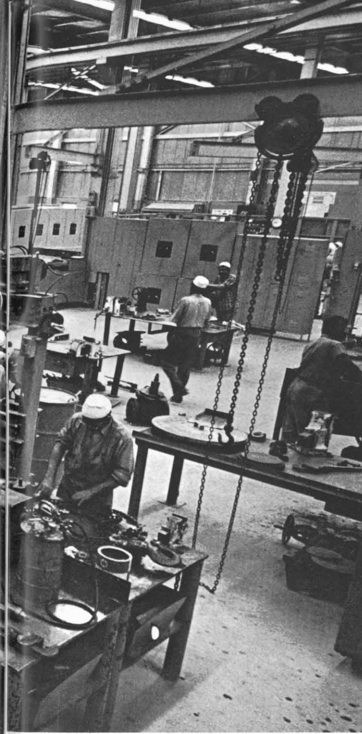
self-propelled cranes on overhead I-beams and chain hoists, above, on pillars.
