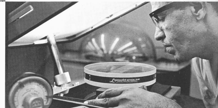
'Abd al-Rahman Genari works with a "lapping" machine which measures flatness with the aid of light waves.
