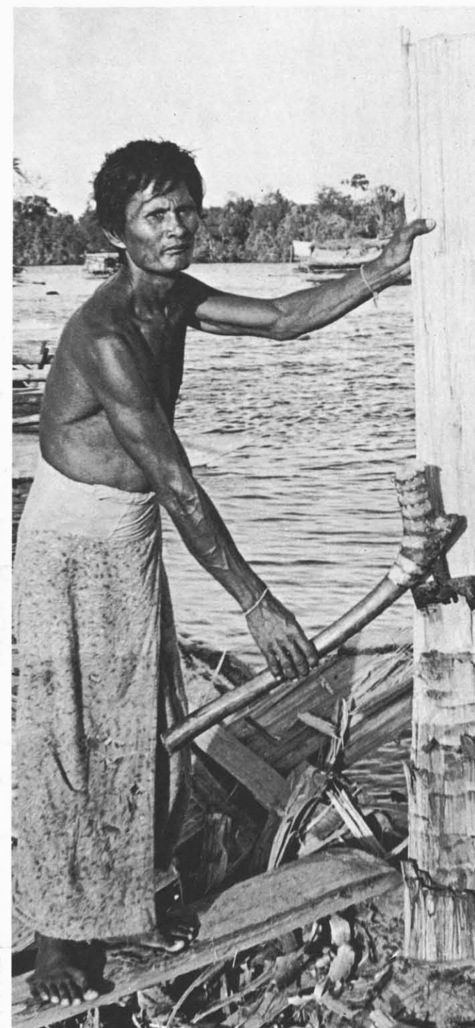
Using a "baliang" (axe), a Badjao carpenter makes usable boards out of driftwood.
