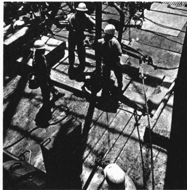
From the floor of the mobile platform, Saudi Arab assistant driller (foreground) and rigmen carefully guide the probing bit to the Gulf floor.
