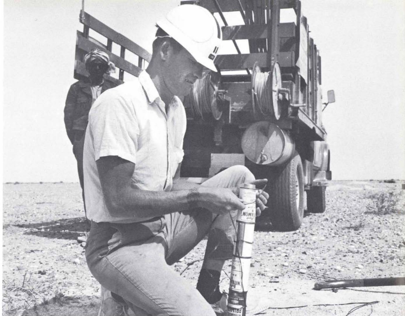
Third in line after surveyors and drillers is shooter E. W. Taylor, who attaches electric wire to a charge of Nitromon prior to lowering charge and wire into the shot hole.
