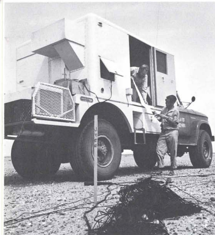
After a charge is fired observers check record of shock wave left on sensitized paper.
