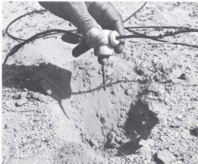
A crewman plants a "geophone" in the ground to eliminate the noise of the wind.
