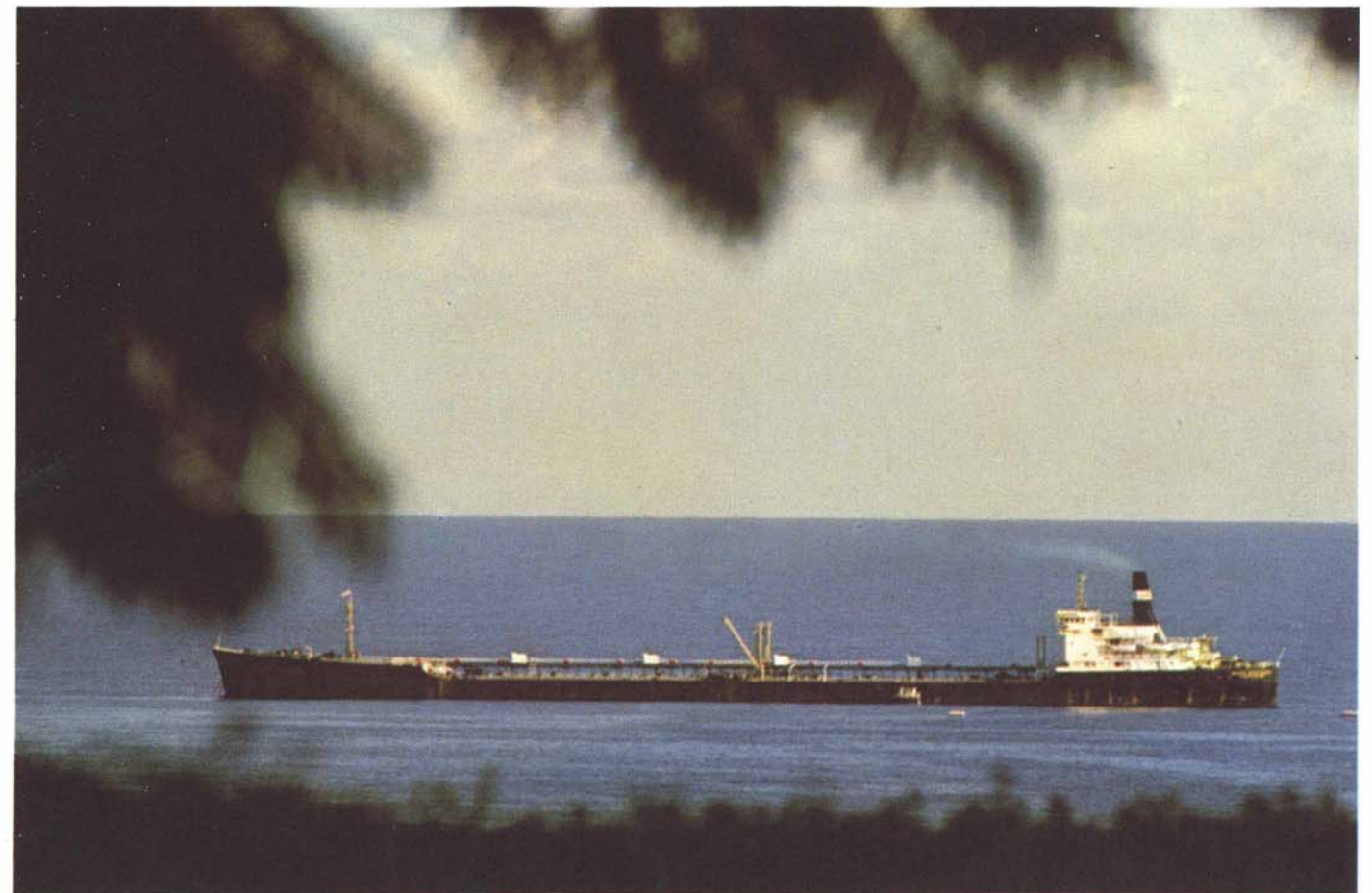
Anchored off the Trans-Arabian Pipe Line Company's terminal at Sidon, Lebanon the Esso Den Haag loads crude oil. The ship can load some 27 million gallons in about 15 hours.
