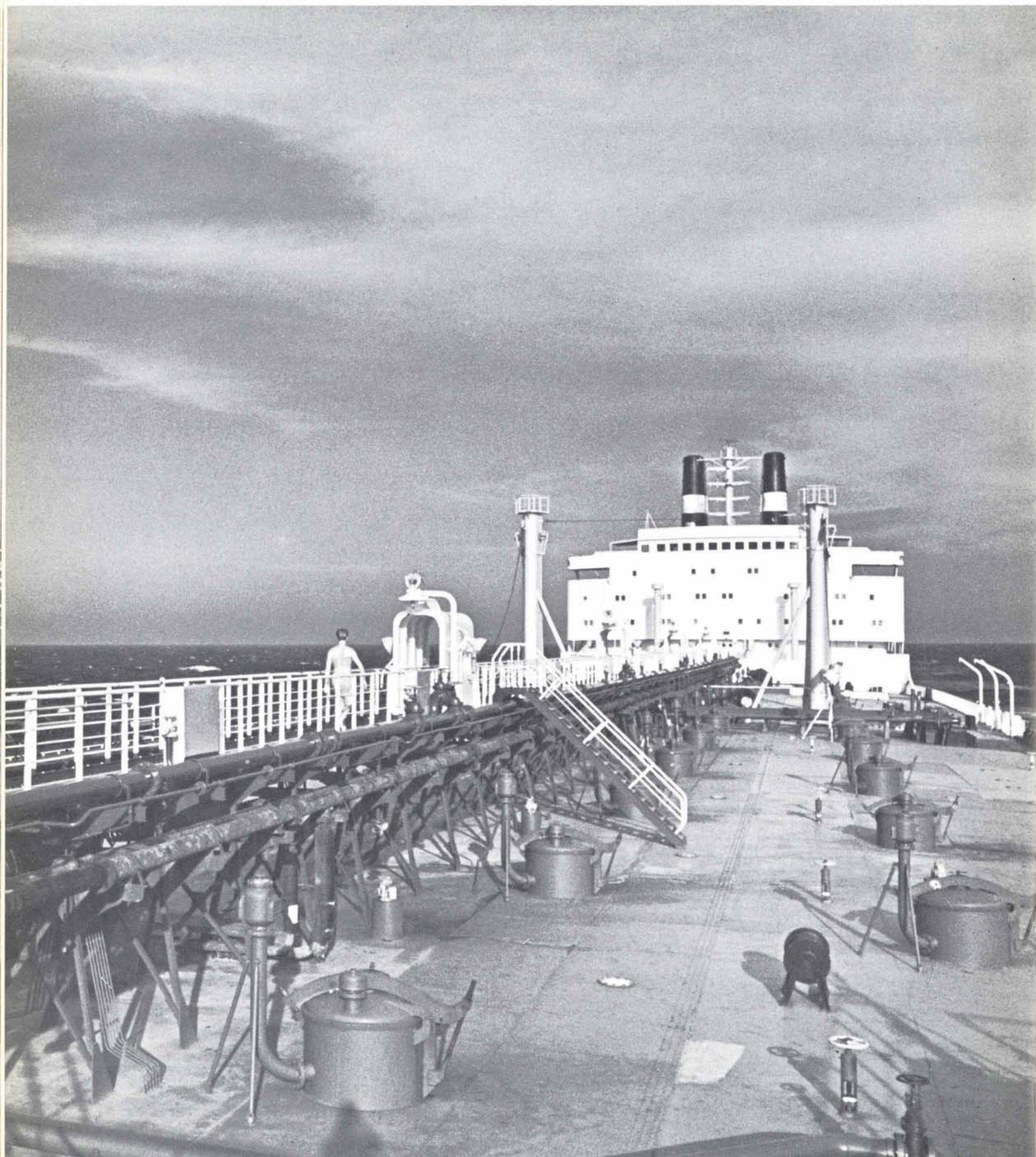
Clustered beneath the fore and aft gangway, the ship's main cargo pipes and steam and water lines stretch from superstructure to forecabin, accenting the ship's already impressive length.
