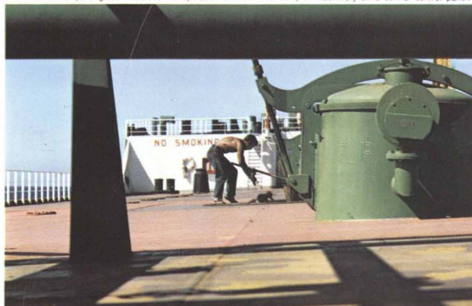
For safety, each of 39 hatch covers is screwed firmly in place by means of a long hatch cover control screw.
