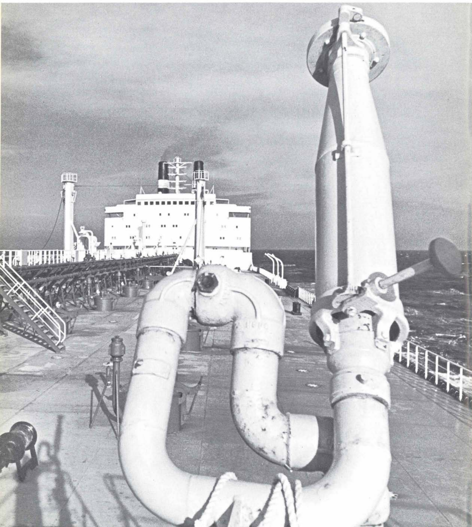
Fire precautions on the Den Haag include eight foam monitors that resemble antiaircraft guns and are positioned so crewmen can spread a canopy of foam and water over the entire main deck area.
