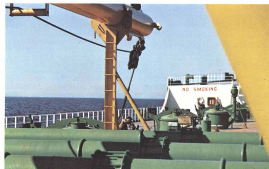
On a tanker the manifold is a battery of pipes through which oil flows aboard and is routed into the tanks.
