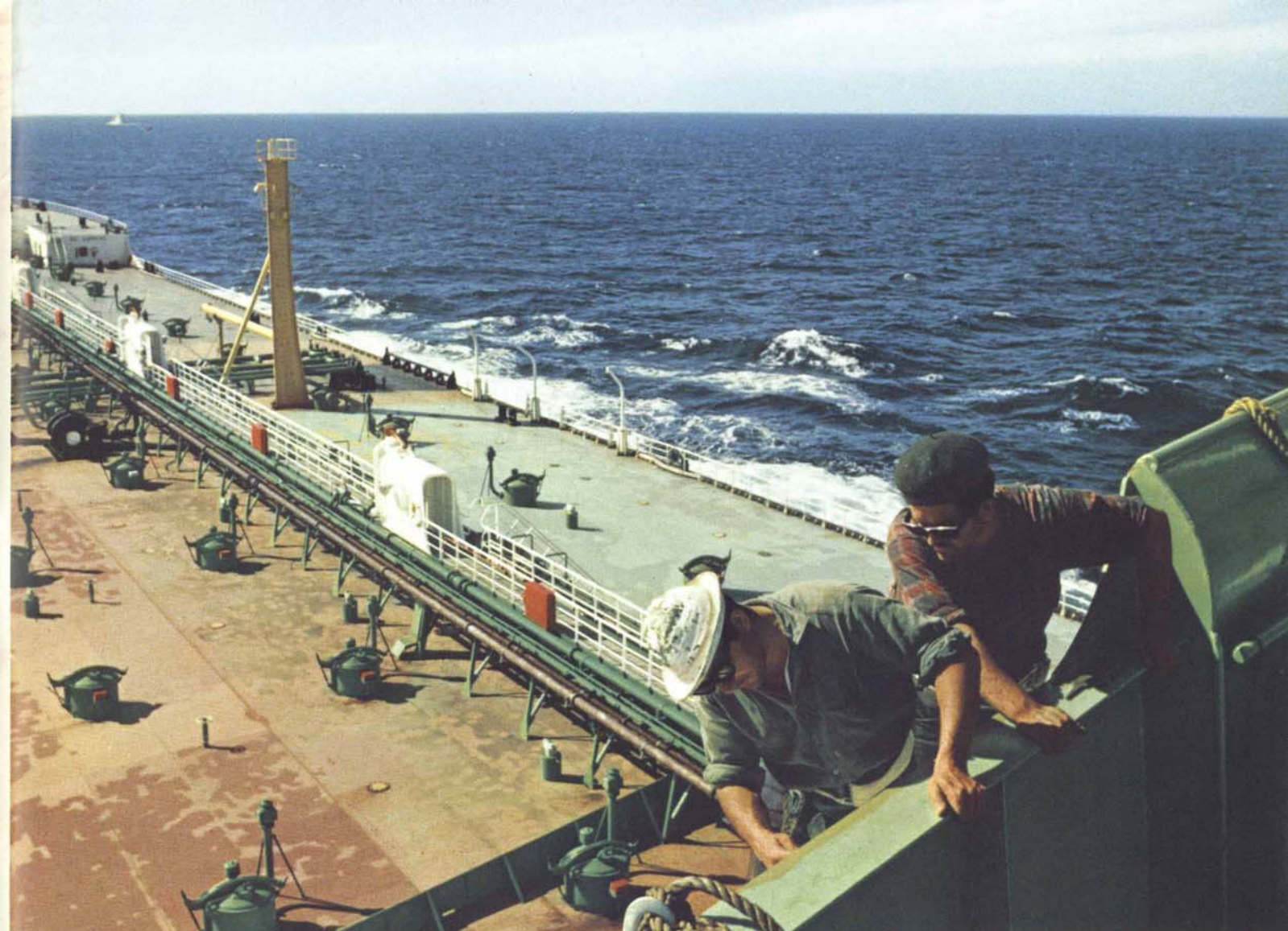
On a scaffolding high on the sheer side of the superstructure seamen ignore the spectacular view as they turn to the never-ending task of the sailor: scraping and repainting corroded metal.
