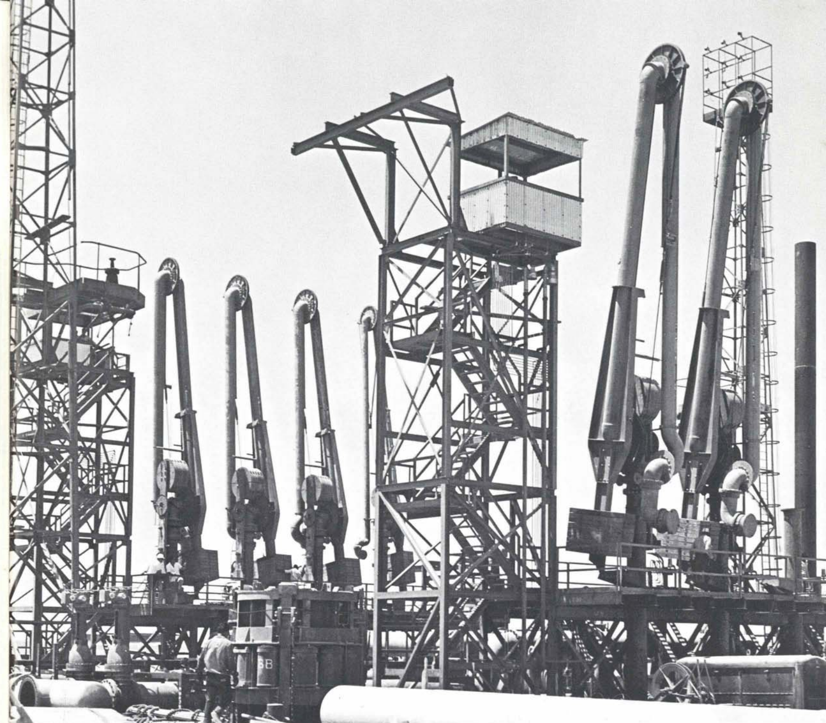
Some of the equipment assembled on Bahrain for Sea Island One, included seven Chiksan loading arms, an operator's control tower and two floodlight towers.
