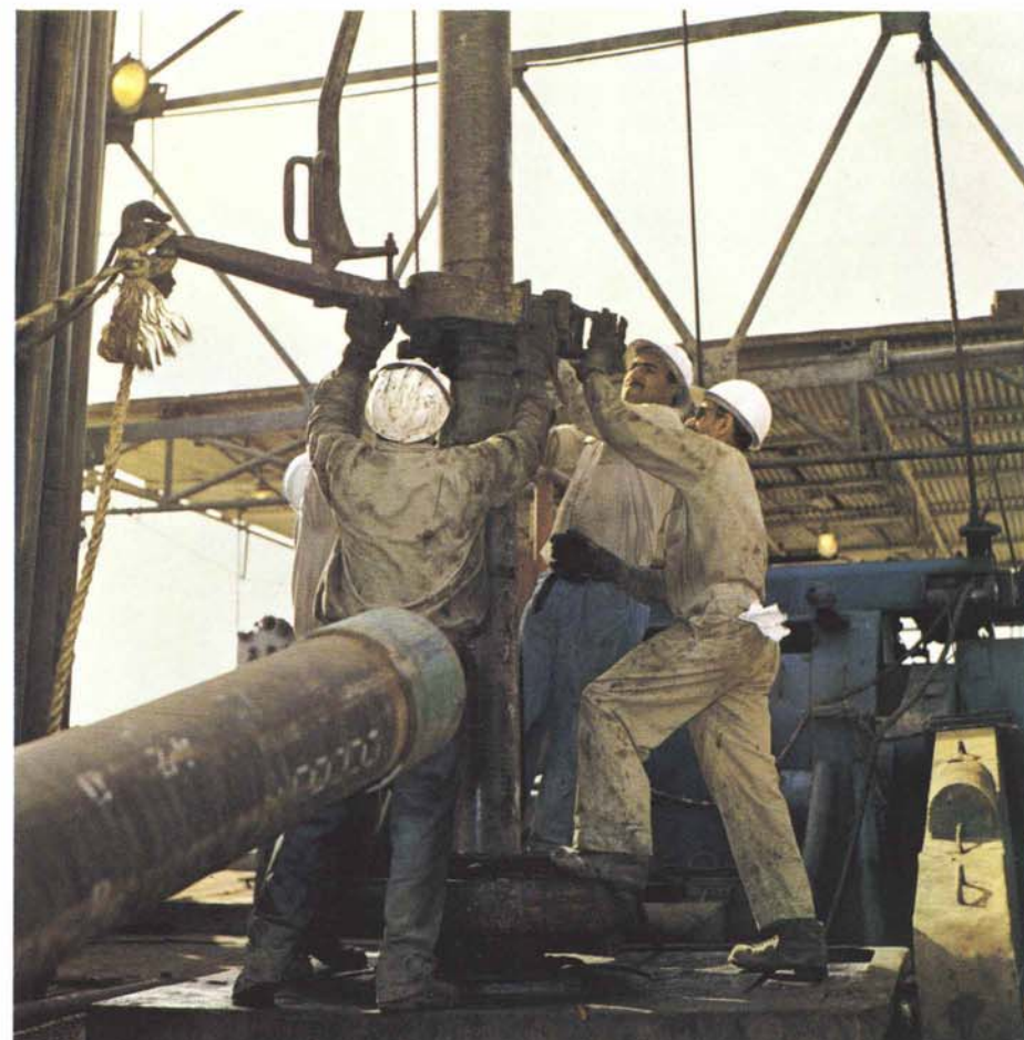
Helmated members of drilling crew attach drill pipe tongs that act like pipe wrenches and are used to unscrew the pipes.
