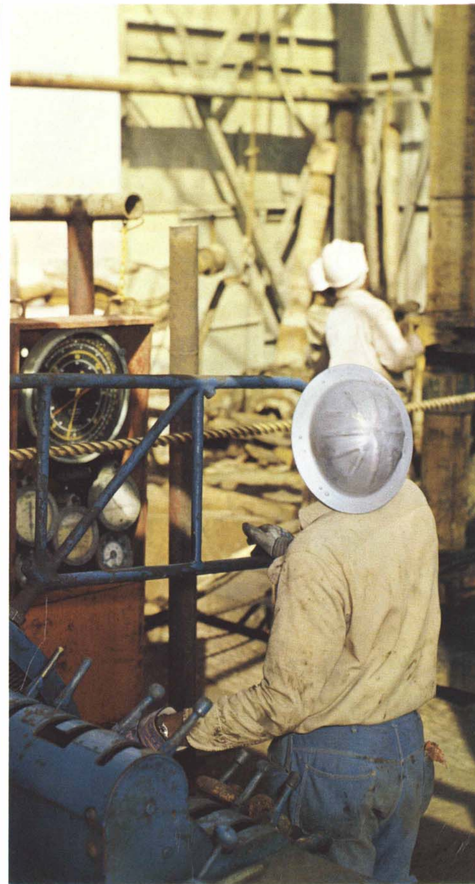
To pull up the drilling string, join and unjoin the lengths of pipe and run the string into the hole, requires power and skill.
