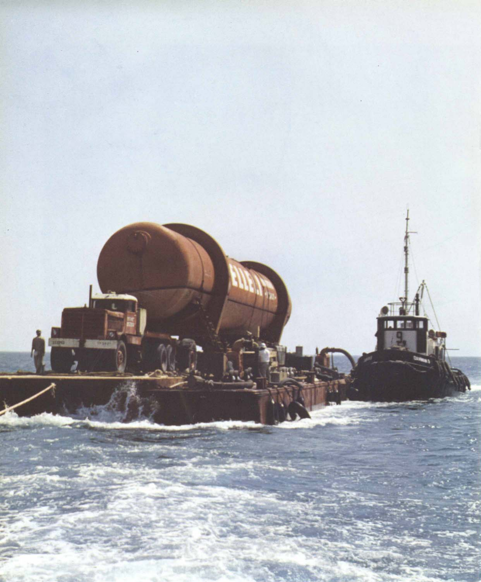
Brought to Saudi Arabia aboard the freighter Kandelfels, the huge steel cylinder was lowered onto the bed of a trailer-truck mounted on a barge and secured to the trailer. The barge was then towed ashore.
