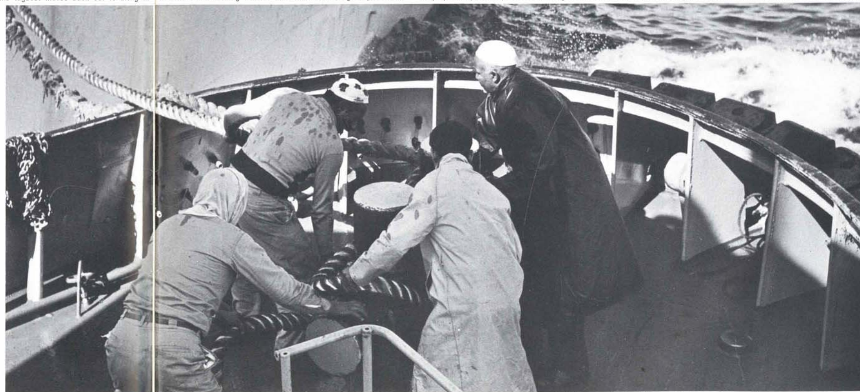
Preparing to take a tanker in tow outside the Ras Tanura harbor, the Abqaiq 4 stands by off the starboard bow while sailors on the ship pull the thick hawser aboard with a smaller line and the tugboat crew fastens it securely.
