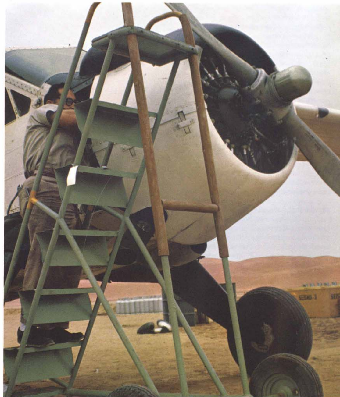
Mechanical supervisors fly to the Sand Mountains regularly to give 100-hour checkups to the Beavers attached to exploration parties there.
