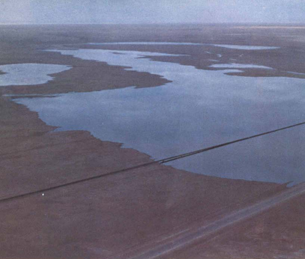
Before repairing the leak the engineers had to first lower the lake level by draining oil and water into pond, at left, and across road.
