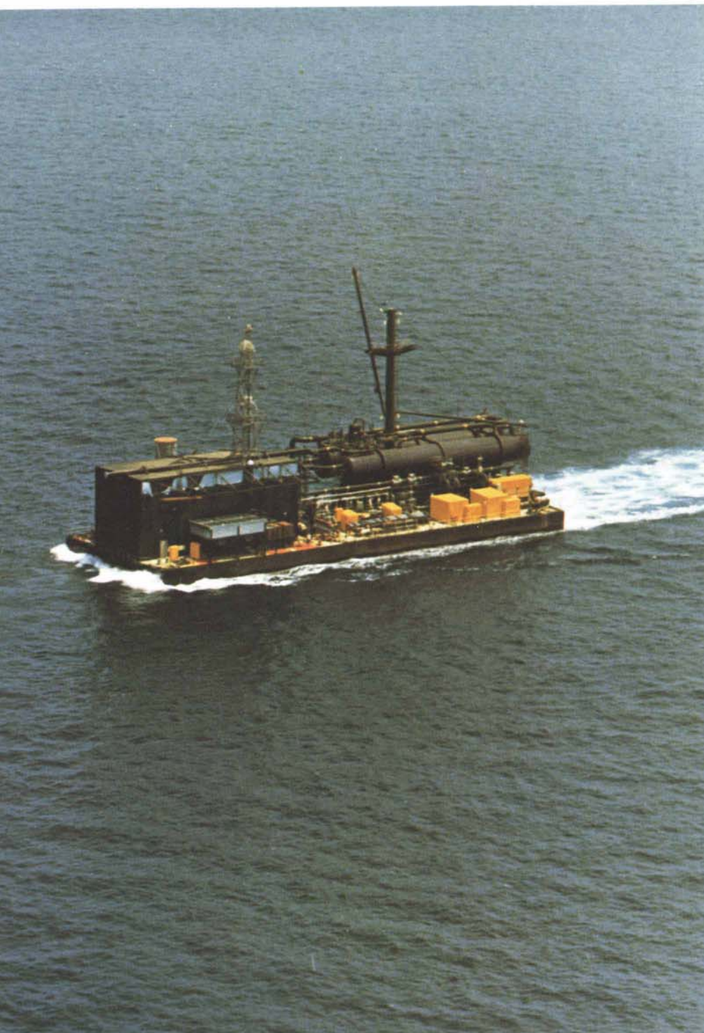
This unusual barge was towed into Safaniya waters from Japan, later cut in two and stood on legs to make Aramco's first offshore GOSP.
