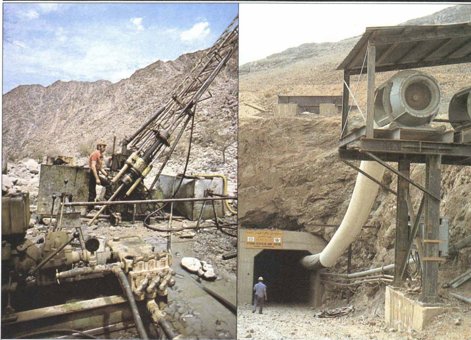
At left: drilling for ore samples is a preliminary in all mineral exploration; at right: great fans force air into a mine shaft at the famous Mahd al-Dhahab.
