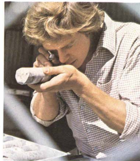
Geologist inspects diamond-drill core sample.
