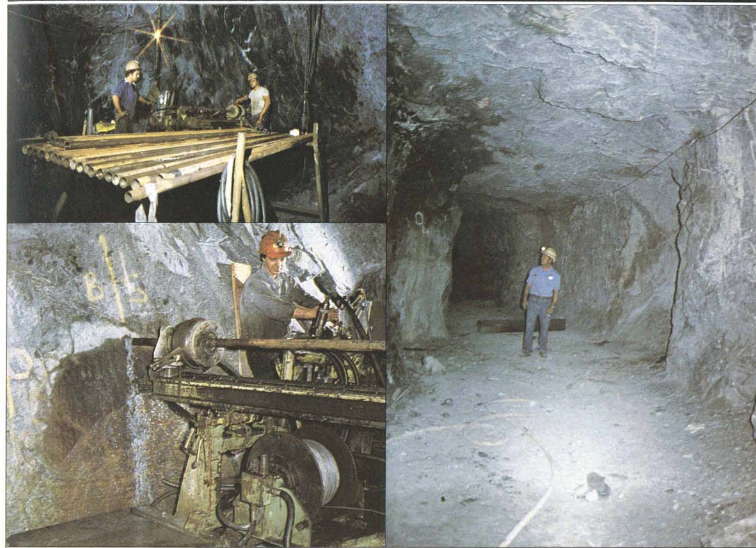
Top and bottom left: in a Wadi-Sa'ada shaft mine workers drill horizontal holes with diamond drilling rigs to get new ore. Above: inside Mahd al-Dhahab.
