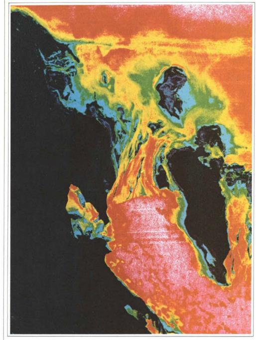
the mapping, classification and evaluation | of sand deposits in upwind areas," says Anton. "It may also be necessary to install sand traps, wind stations, tracers and piezometers. One single shamal season often one single sand storm caused by those fierce northerly winds - can give an idea of local sand paths, information needed for detailed designs of roads, power lines, runways, communities and industrial plants."
