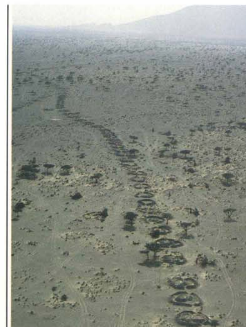
Telltale tops of access shafts to an underground falaj.
