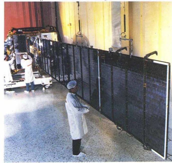
Power-providing solar wings being fitted to the Arab communications satellite.
