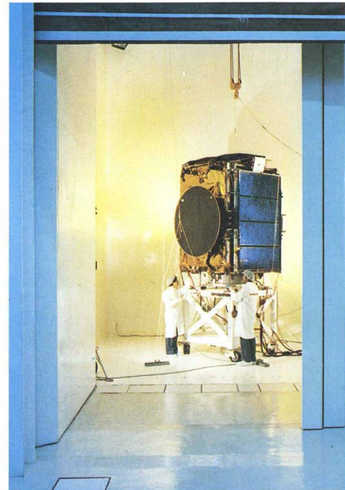
Arabsat-A during tests in a launch-simulating chamber in Cannes, France.
