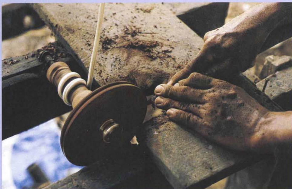
To craft a Kelantan top, the core disk of hardwood is prepared on an ingeniously devised treadle-powered bow lathe. The cord runs up from the treadle, around the spindle and up to a bicycle innertube fixed overhead. The treadle powers the downstroke and the innertube's elasticity powers the return stroke. The groove around the core's circumference will allow the lead casting to grip the wood firmly.
