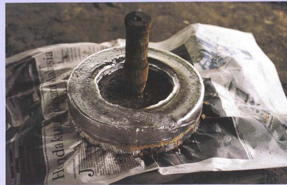
The lead casting, thicker than the top's hardwood disk, is allowed to cool before it goes back to the lathe. The thick wooden spindle will be removed when the lathe-work is done, and replaced with a decoratively tooled, pencil-thin finial made of brass or—on the best tops—of sterling silver.
