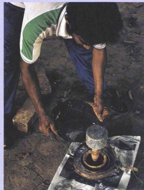
Molten lead—recycled from retired competition tops and from old automobile batteries—is poured into a mold made of a section of tin can and built around the top's wooden core.
