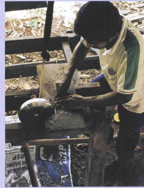
At the lathe again, the maker shapes and balances the lead "tire." A sheet of newspaper below the lathe collects lead shavings for reuse.
