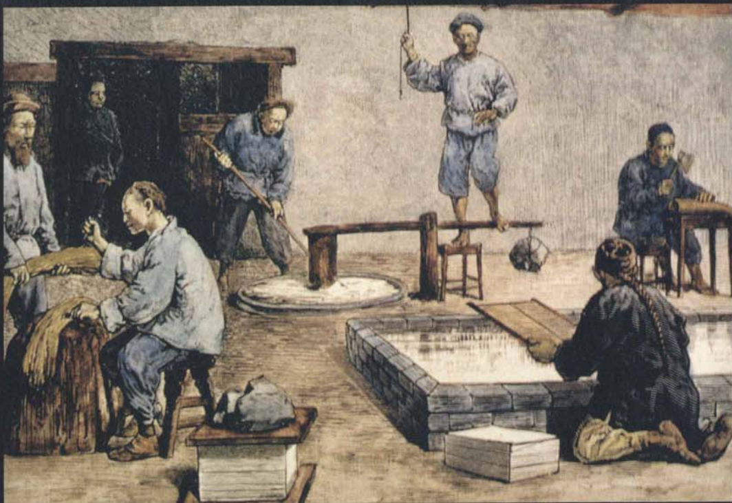
In this modern depiction of an early Chinese paper mill, strips of mulberry bark are scraped (left) and then chopped (background right). The pieces are then pounded into pulp with a counter-weighted step-hammer (background center) and the pulp is stirred into a water-filled vat. The single-screen moulds were hand-dipped, and the resulting sheets were dried under pressure (foreground). Below: A Chinese paper mould dating to the first century.
