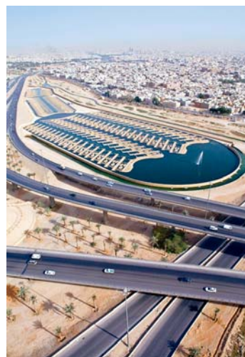
Above: This bilingual map shows the middle 50 kilometers (35 mi) of Wadi Hanifah, along with major features of the 10-year project. Left: Aerial views of the upper wadi, which is dry except during winter rains, and the three-pond, 134-cell bioremediation facility, which produces water safe for human contact at one-third the cost of a mechanical treatment plant.
