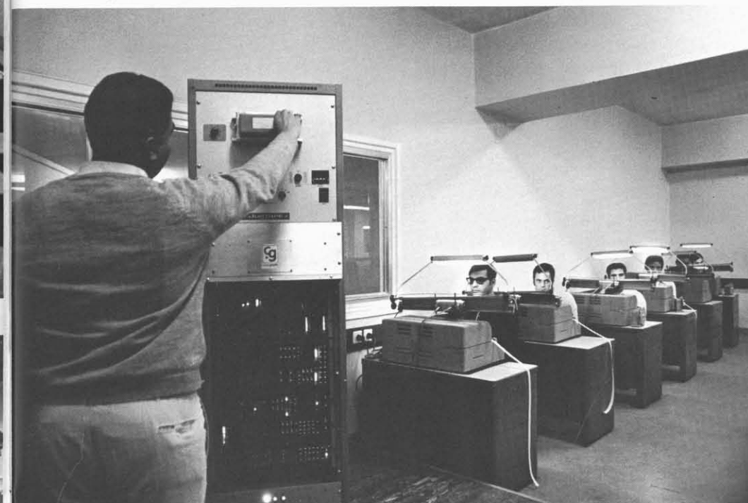
Operators feed stories into IBM computer programmed in Arabic and hooked to electronic Linotype machine capable of setting 1000 lines per hour. The electronic photo-scanner is in the auto-engraving section.
