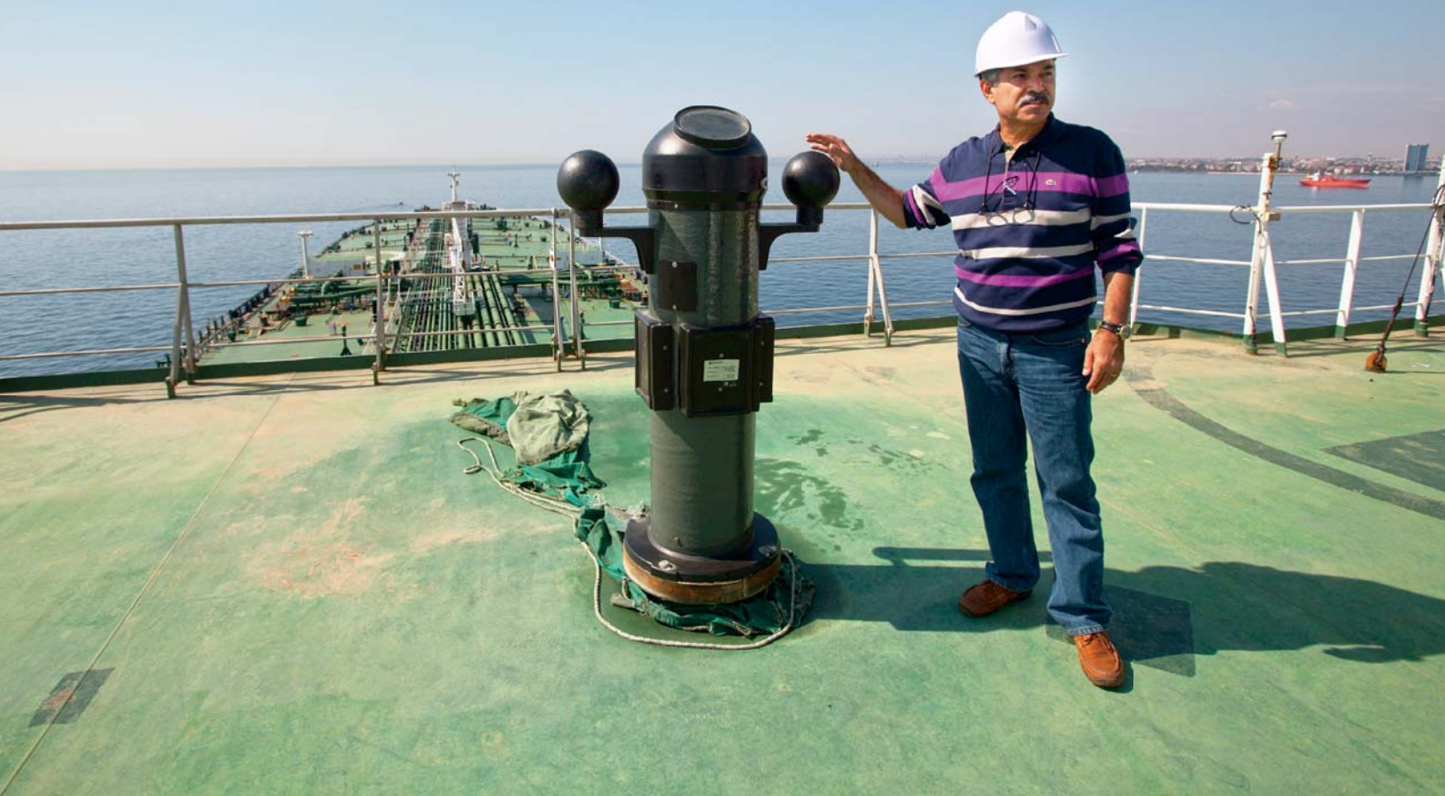
Standing by one of the two magnetic compasses that back up electronic navigation equipment aboard the M/T Ottoman Nobility , Captain Tuğrul Vural is chief marine superintendent for Güngen Maritime and Trading of Istanbul, which owns four tanker vessels. Preceding spread: The M/T Ottoman Nobility enters the Bosphorus heading due north at some six or seven knots, carefully slipping its 269-meter length between European Istanbul on the left and Asian Istanbul on the right. The Maiden's Tower is visible at upper right.
