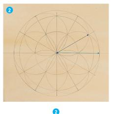
Draw two encompassing circles by placing the compass point in the center, and open the compass to the intersections indicated.
