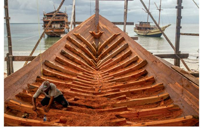
A craftsman scrapes sawdust where ribs meet hull planks on a *pinisi* boat under construction in Tana Beru, where Haji Abdul Wahab, **RIGHT**, has been building the iconic Indonesian schooners for more than 30 years.
