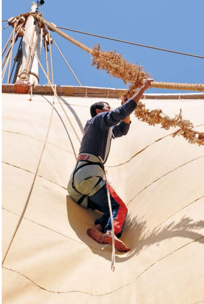
A crewmember wraps protective baggywrinkle on the manila-fiber rigging where it might wear holes in the sails made of woven palm fronds.
