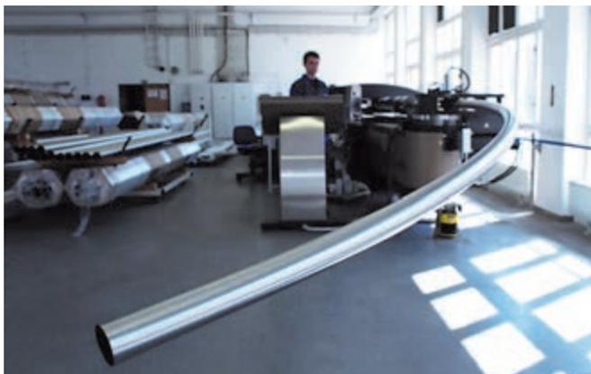
**Above:** A five-ton composite wooden beam, glued and laminated and bent to twist 90 degrees, gets wheeled into a warehouse in Germany before shipping to Ithra. **Lower:** One of the 93,403 stainless steel cladding tubes is shaped to its individual specifications using a custom-built fabricator.
