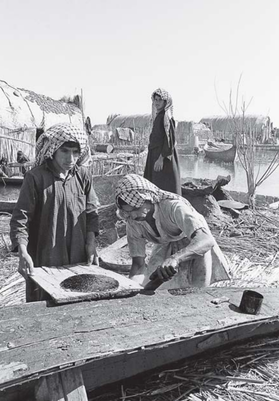
A villager applies thick bitumen, purchased with the proceeds of fish and reed-mat sales to Iraqis outside the Marshes, to seal a mashuf in Al-Sahein village.
